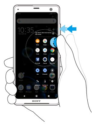
• To activate the **Side sense menu**, double-tap the side of the device.
