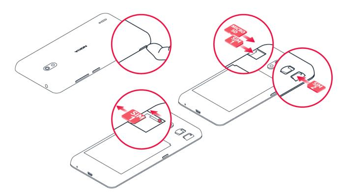
1. With the phone facing down, put your fingernail in the slot on the side of the phone, bend the back cover open, and remove it.
