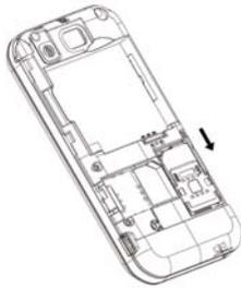
2 **Note:** pushing the SIM card carefully with the metal surface downwards and move it into the groove of the
