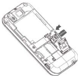
**NOTE:** Pushing the T-Flash card carefully with the metal surface downwards and move it into the groove of the T-Flash card holder.
