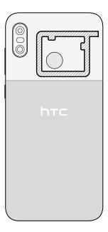
Make sure that the NFC area (shaded part) of HTC U12 life and the other phone's NFC area are close to one another. Experiment by slightly moving the phones until a connection is made.
