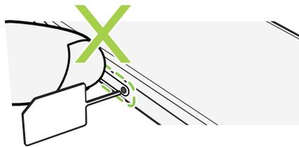
3. Push the tip all the way into the hole until the tray ejects, and then pull the tray out.
