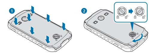
Ensure that the back cover is completely closed and the screw is tightly fastened to avoid water damage.
