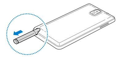
When you pull out the S Pen from the slot, the device detects it and performs the following:
