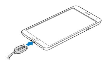
When using a USB 2.0 cable, plug the USB cable into the right side of the multipurpose jack as shown in the image below.
