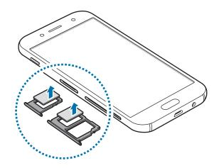
4 Insert the SIM card tray back into the tray slot.
