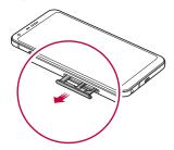
3 Put the SIM card on the card tray with the gold-coloured contacts facing downwards.
