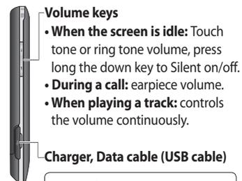
**TIP:** Before connecting the USB cable, wait until the phone has powered up and has registered on the network.
