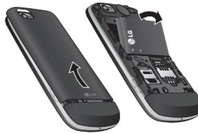
**⚠ WARNING:** Do not remove the battery when the phone is switched on, as this may damage the phone.
